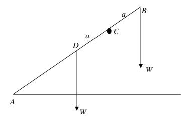
Using the 3 – force result, the total reaction S must pass through C as well.
