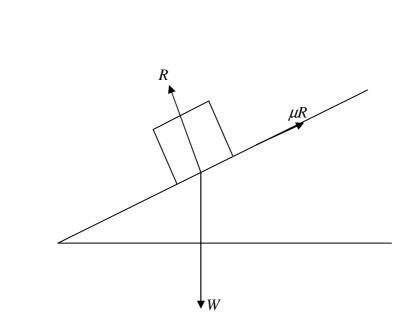
Since the lines of action of the weight and the friction are fixed, then using the 3 - force result, the line of action of the reaction passes through the intersection of the other two.
