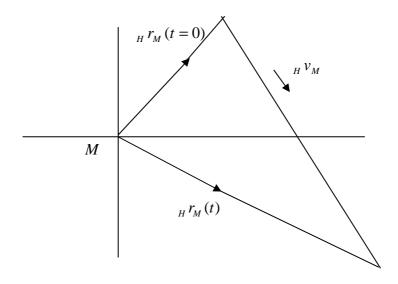
Closest approach occurs when  $_{H}r_{M}(t)$  is perpendicular to  $_{H}v_{M}(t)$
