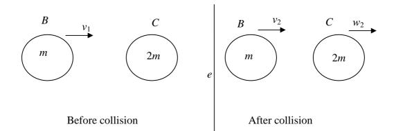
$$e = \frac{w_2 - v_2}{v_1 - 0} \implies w_2 - v_2 = ev_1$$
