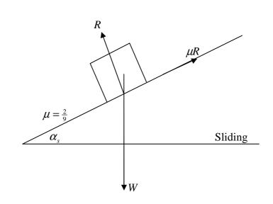
Resolving vertically:  $R = W \cos \alpha_s$  ...(a) Resolving horizontally:  $\mu R = W \sin \alpha_s$  ...(b)
