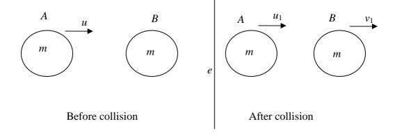
$e = \frac{\text{SeparationSpeed}}{\text{ApproachSpeed}} = \frac{v_1 - u_1}{u - 0} \implies v_1 - u_1 = eu \quad \dots (a)$
